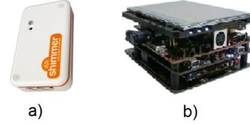
Fig. 3: a) Shimmer node, b) gateway
